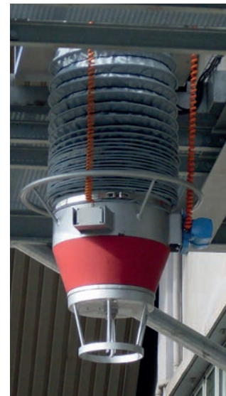
mechanical cleaning and loader filter
