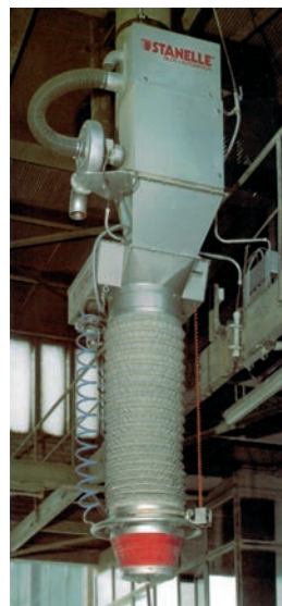
Complete solution with pneumatic cleaning and loader filter
